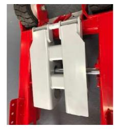
The lifting-bar and rollers, located underneath the platform, slide in the platform's slot, as required.
