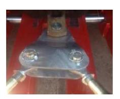
The two toplinks (which are adjustable in length) connect between the hitch-couple, and the most appropriate spare opening in the support stands.
