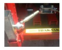
When the connections are secure, the anchor pins can be withdrawn from the fixing brackets.
