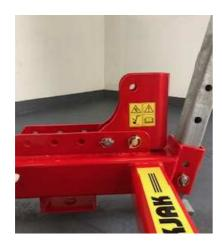
The linear position of the link fixing brackets is adjustable to accommodate different tractor sizes
