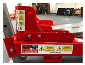
11. Remove the lock- pins from the lower-link fixing brackets.
